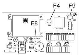
In case of overload or short circuiting at the relay outputs, fuse F9 is triggered (if the power for the external consumers is supplied from terminals "I" of "n").
