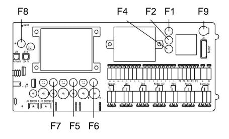
Fuses Testomat 2000<sup>®</sup> Fuses Testomat ECO®
