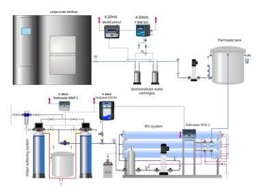
Surgical instruments can be destroyed by silicates > 1ppm in the sterilization steam. The silicate monitoring with the Testomat<sup>®</sup> 808 SIO2 helps to eliminate this risk and in the long term to avoid the high costs of replacement of surgical instruments.
