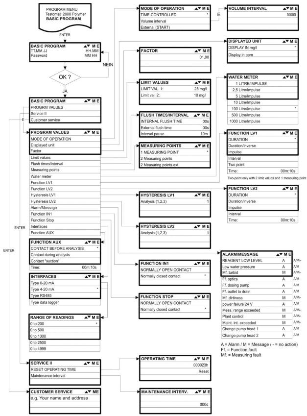
Call the basic factory program by simultaneously pressing and holding down the "M" and "i" keys while switching on the instrument. CAUTION, the last set of programming will be erased!
