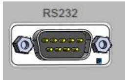
The serial interface RS232 is located at the front of Testomat® 808 (after opening the housing cover). Use a ribbon cable with a 9-pole Sub-D connector to connect the plug J3 on the controller board to RS232. Use this RS232 interface to connect a computer/notebook to the controller board of Testomat® 808 via a null modem cable and update the instrument's firmware.
