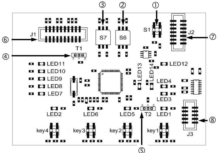
Keys 1 to 4 are located at the front of the board. Please refer to the section entitled “[Functions of the operating and display elements](#)” on page 11 for a detailed description of its operating system and the display elements.
