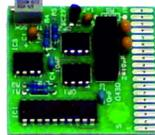
Add a 0–10 V or 2–10 V voltage output to Testomat 2000®.
