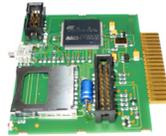
Use the SD Card Data Logger to save measuring results and error messages for up to 10 years.
